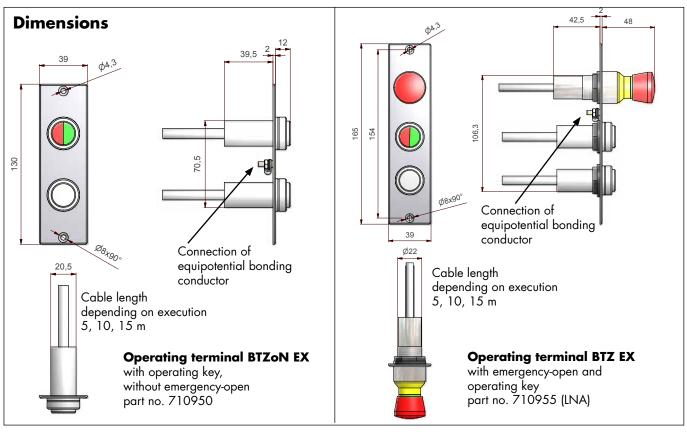
The operating terminal EX is available with and without emergency-open switch. The type with emergency-open is slightly longer. Its front plate measures 165 mm instead of the 130 mm of the type without emergency-open switch. The emergency-open switch on a terminal unlocks only the respective door (LNA).
