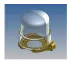
In case the emergency-open switches in an interlock control system are again and again misused, they can be protected by a cover that is prepared for a lead seal (part no. 710839). This cover can be retrofitted and is from transparent, UV resistant plastics with a yellow collar for fixing.
