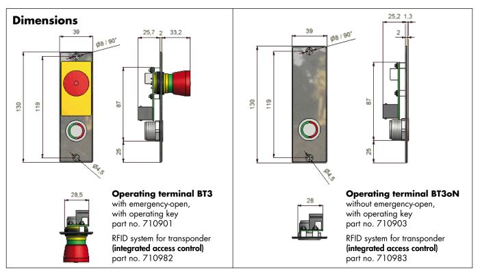
The operating terminal BT3 is connected to the operating terminal BTZ by the connection cable with RJ45 connector (marked yellow). The cable has to be ordered separately. By default two lengths are available:
