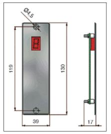
from 9 to 0, thus indicating the remaining time during which the doors stay locked.
