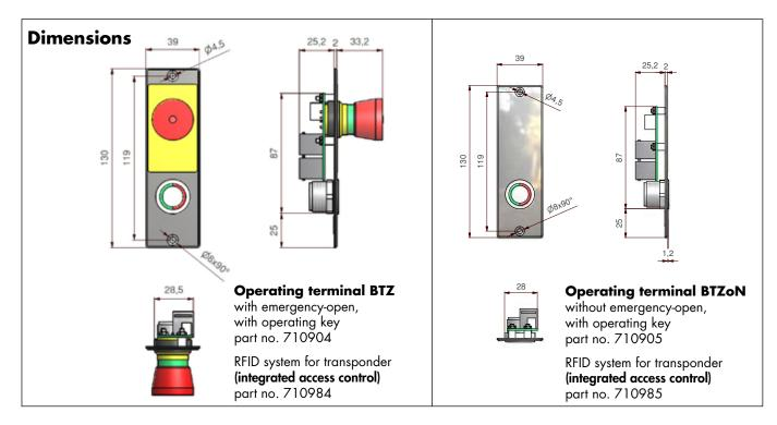
The DICTATOR terminals meet the requirements of clean rooms. The operating terminal BTZ is available with and without emergency-open switch.
