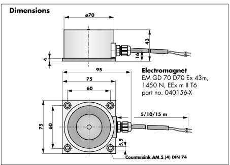
To accomplish the mounting every magnet needs a potential equalisation. On the mounting plates is provided a connection for connecting an equipotential bonding conductor (to be provided on site).
