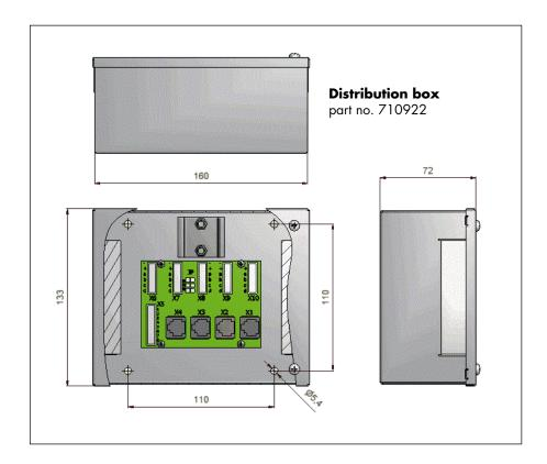
The strain relief of the incoming and outgoing cables is achieved by fixing the cables with tie wraps to the two cable support brackets. The cable inlets are sealed dust proof by cellular material.
